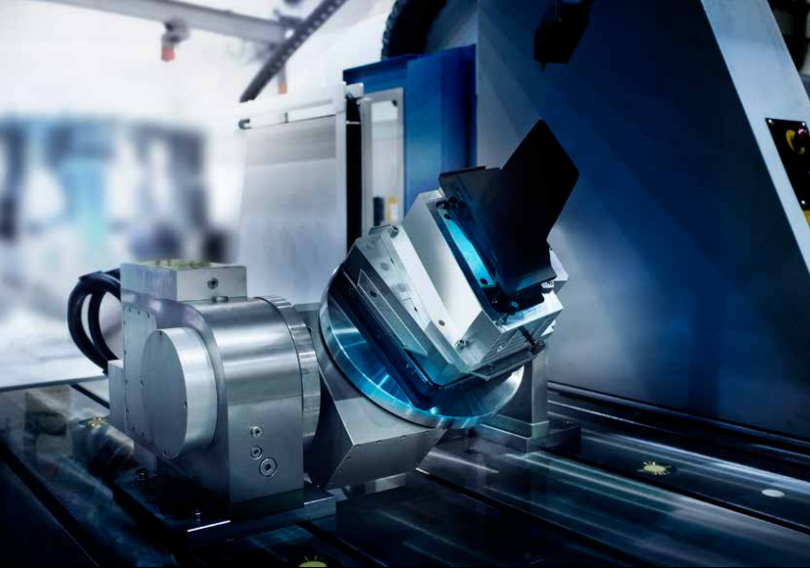
5 th /6 th axis as fully integrated EDM axes for machining high-precision components of different sizes
