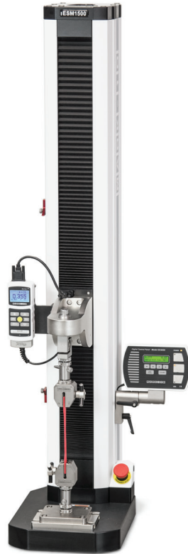
ESM1500 1,500 lbF [6.7 kN] 32 in [813 mm] travel
