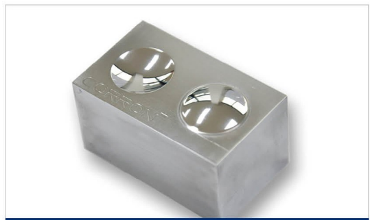
Single crystal diamond tool mirror machining
