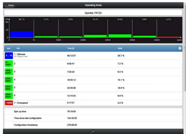
Duration of operation in different speed ranges display of the configurable operating hours counter in the MiniCODER plus
