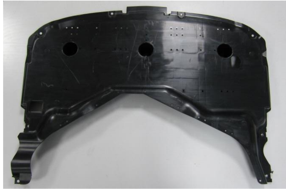
NAME : Under Cover MATERIAL : PP COMPANY : MAZDA
