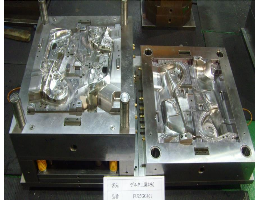
NAME : Seat Side Cover 金型 MATERIAL : KP4M (P20) COMPANY : DELTA KOGYO (MAZDA)
