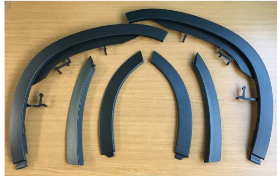
NAME : Side Garnish MATERIAL : PP COMPANY : SUBARU
